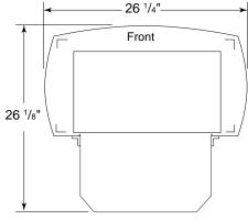
Figure 5 - Stove With Burner System Bottom Dimensions
